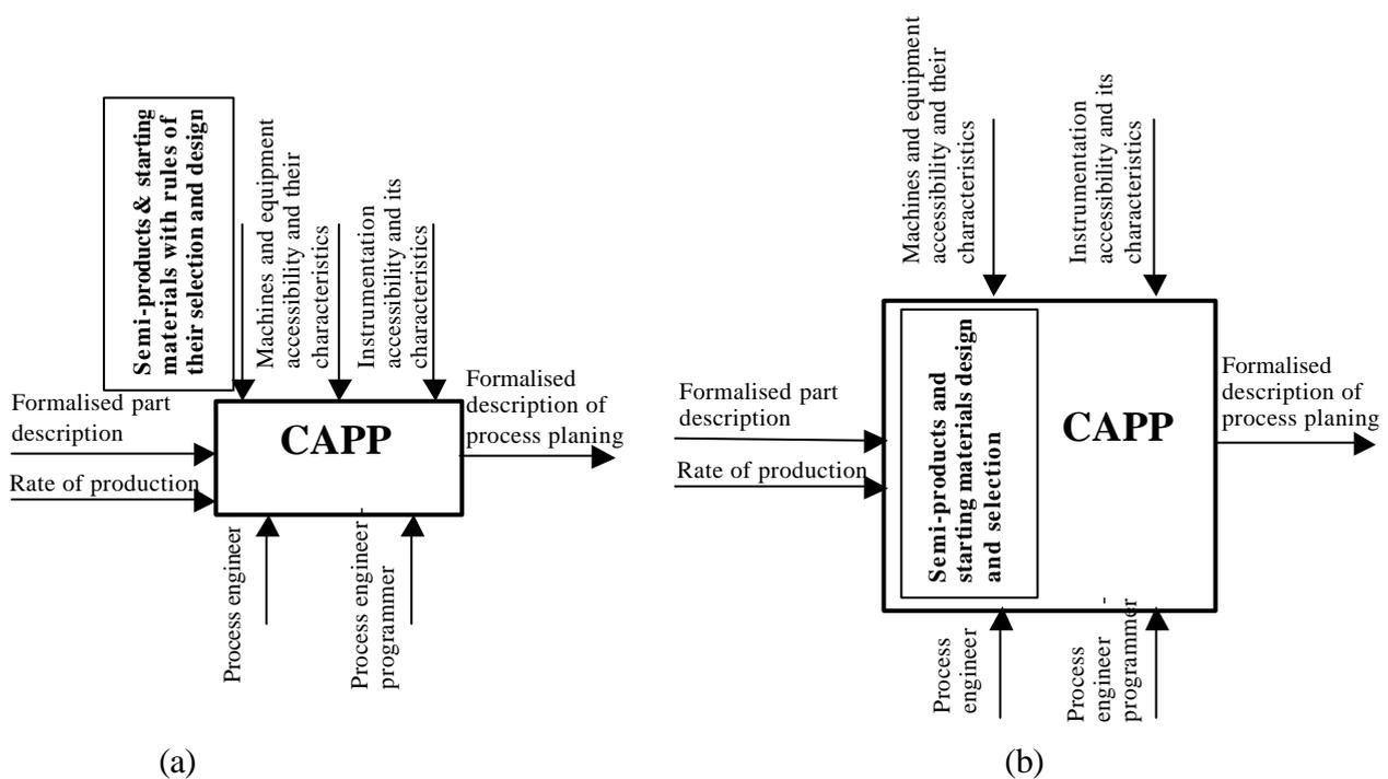
Fig.1. Computer aided semi-product selection and design position in the CAPP process currently applied [10] (a) and in the proposed system (b).
