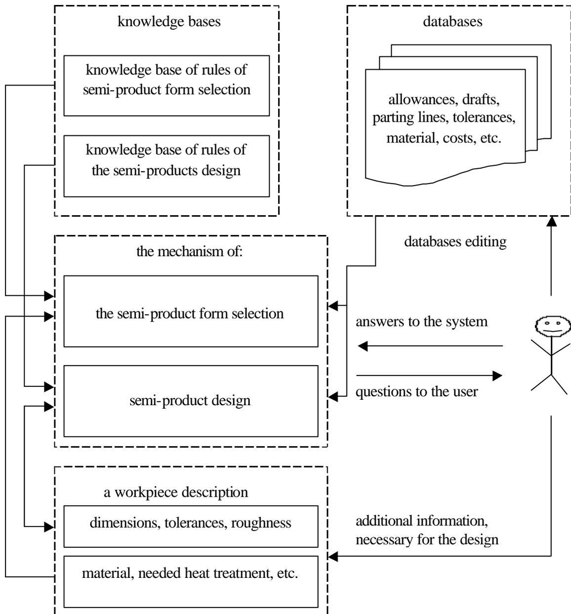
Fig.2. Diagram of the conception of the computer aided semi-products selection and design system.
