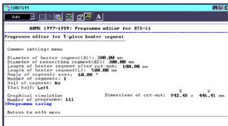
Fig. 3 Dialogue window of program EDBTS11 for entering of input data
