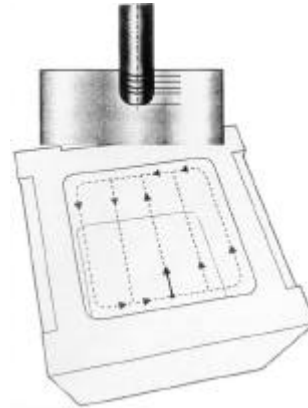
Fig. 6. Example of machining with a ball nose endmill [2].
