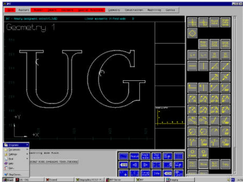
Figure 2: Computer aided manufacturing in the area of water jet cutting (Unigraphics)
